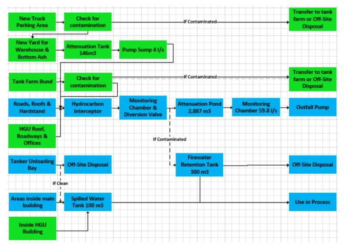
Figure 4. Proposed Stormwater Drainage System Flow Diagram.
