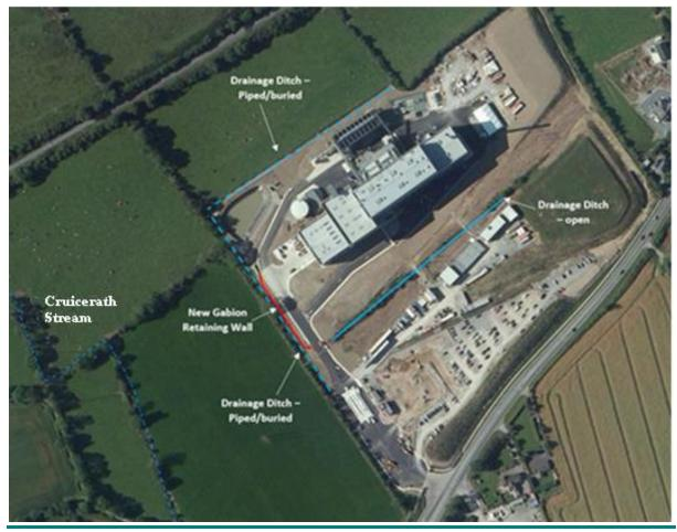
Figure 10: Location of drainage ditches on site
